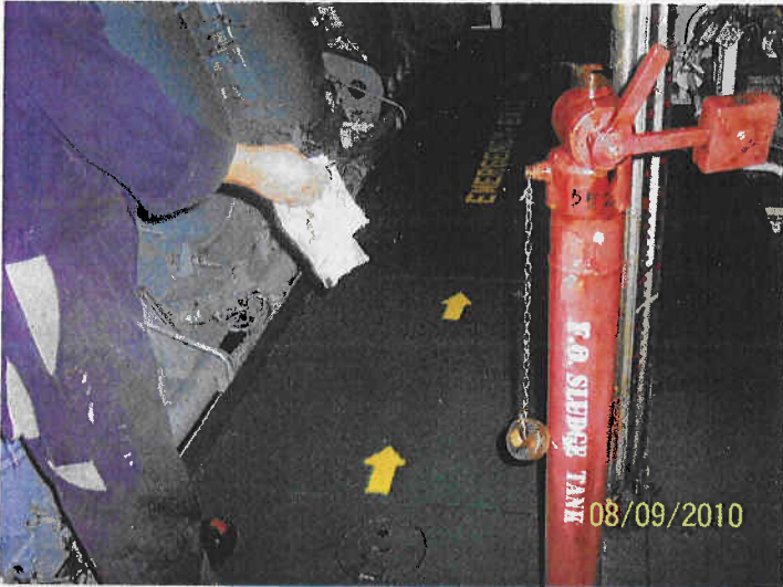
9/8/2010 19 Manual sounding FO sludge tank.JPG
