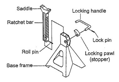
Doc. #302-4 at 72 fig. 1. The model 50163 jack stand includes a pyramidal base frame and a retractable ratchet bar rising from the frame that can support a heavy object. *See id.* at 72–73. The ratchet bar has a number of "teeth" that fit against the pawl. *Ibid.* Ordinarily, a ratchet bar tooth should rest firmly in place against the pawl's body. *Id.* 72–73.
