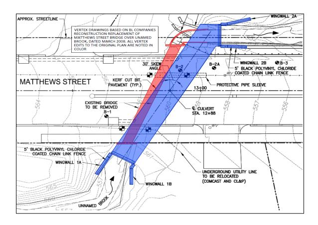
Vertex Comparison, ECF No. 104-32 at 12 (highlighting prior culvert in red and new culvert in blue); Laviero Dep., ECF No. 104-22, 148:2–10. The new culvert was consistent with BL's design: a 9' x 6' precast concrete box with a chain link fence:
